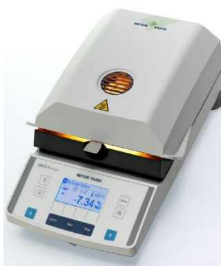
Figure 2.1: Thermobalance Mettler Toledo HB43-S for analysis of water content in the material.
