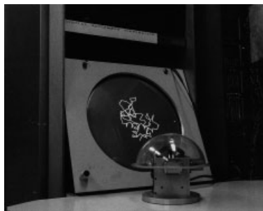
Figure 2-122. The first dynamic molecular display of small molecules by Levinthal was driven by the “Crystal Ball” [193].
